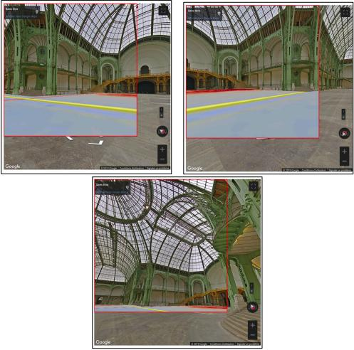
Figure 5, SVO of the ground concentration field due to fictitious release within the Grand Palais building, seen using various PoV
